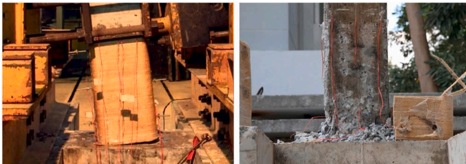
Fig. 25. Structural applications incorporating natural sisal and jute fibre high-strength components, reproduced under license number 5491300556102 from [171].
