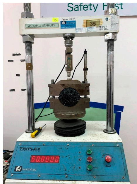
Figure 3. Marshall stability test.
