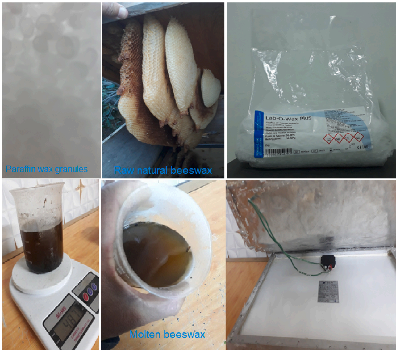
Fig. 3. Preparing PCM panels.
