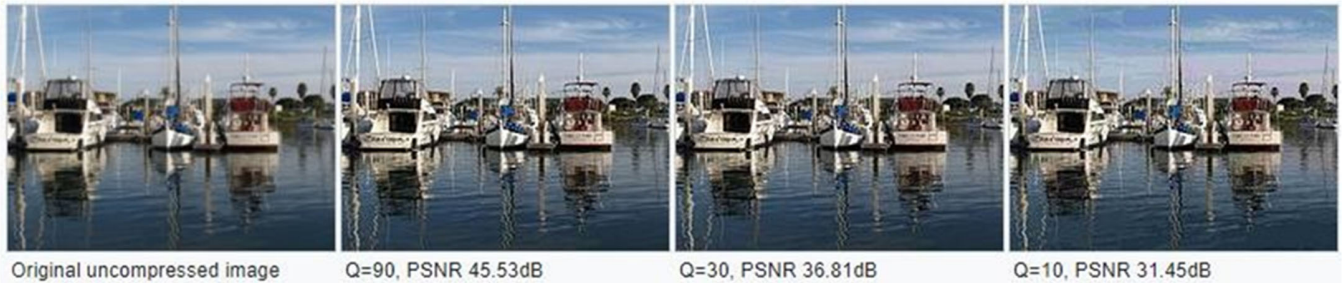
Fig. 9. PSNR values for different quality levels of a jpeg compressed picture
