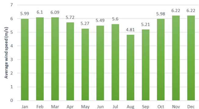
Figure 3. Monthly average wind speeds at a height of 50 m at Zhanjiang port are collected consistently every month of the year.
