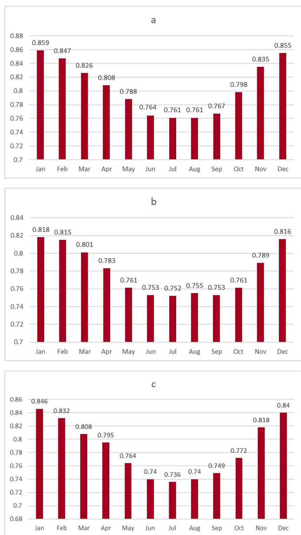
Figure 8. (a) PR for Eqlid. (b) PR for Lamerd. (c) PR for Shiraz (Scenario 1: No tracking system).
