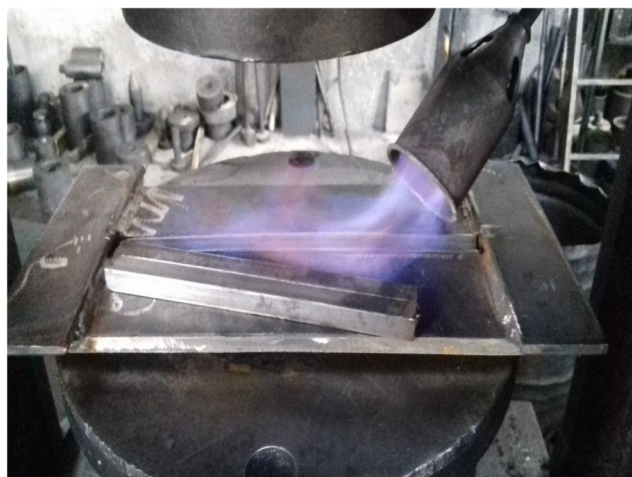
Fig. 4 Warming of the bottom mold to start the APB process
