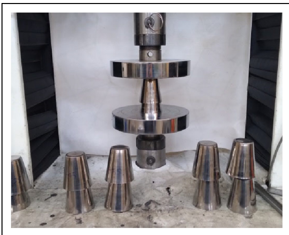
Figure 4. Placement of the samples in the machine to perform the quasi-static compression test.
